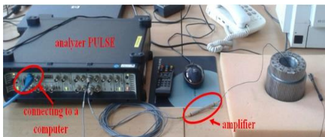
Fig. 1. A set for measuring natural frequencies of the wheel.
