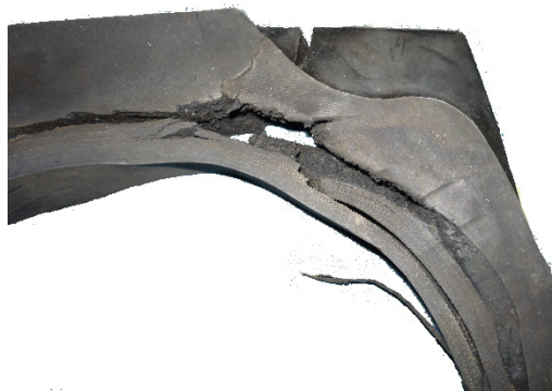
Fig. 2: Destroyed tyre due to the initial cracks in the belt region
