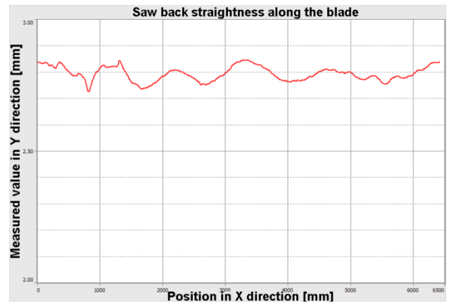
Fig. 17. The graph of saw back straightness along the blade.
