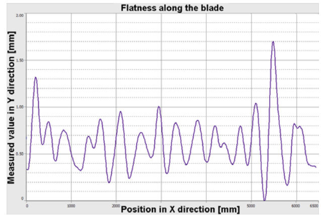
Fig. 16 The graph of flatness along the blade.
