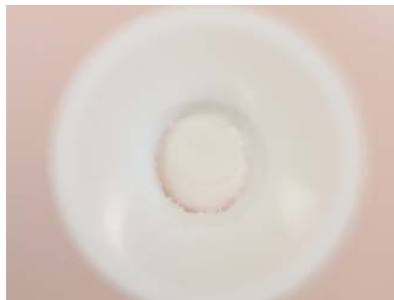
Fig. 9. PP deformation after-drop weight impact test at 230 J.
