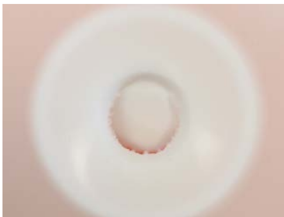
Fig. 7. PP deformation after drop-weight impact test at 100 J.
