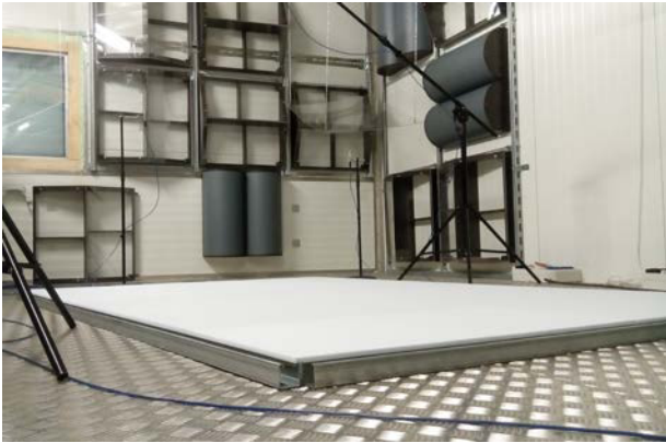
Fig. 3. Measurement of sound absorption of sample 2 in reverberation chamber at TBU in Zlin.
