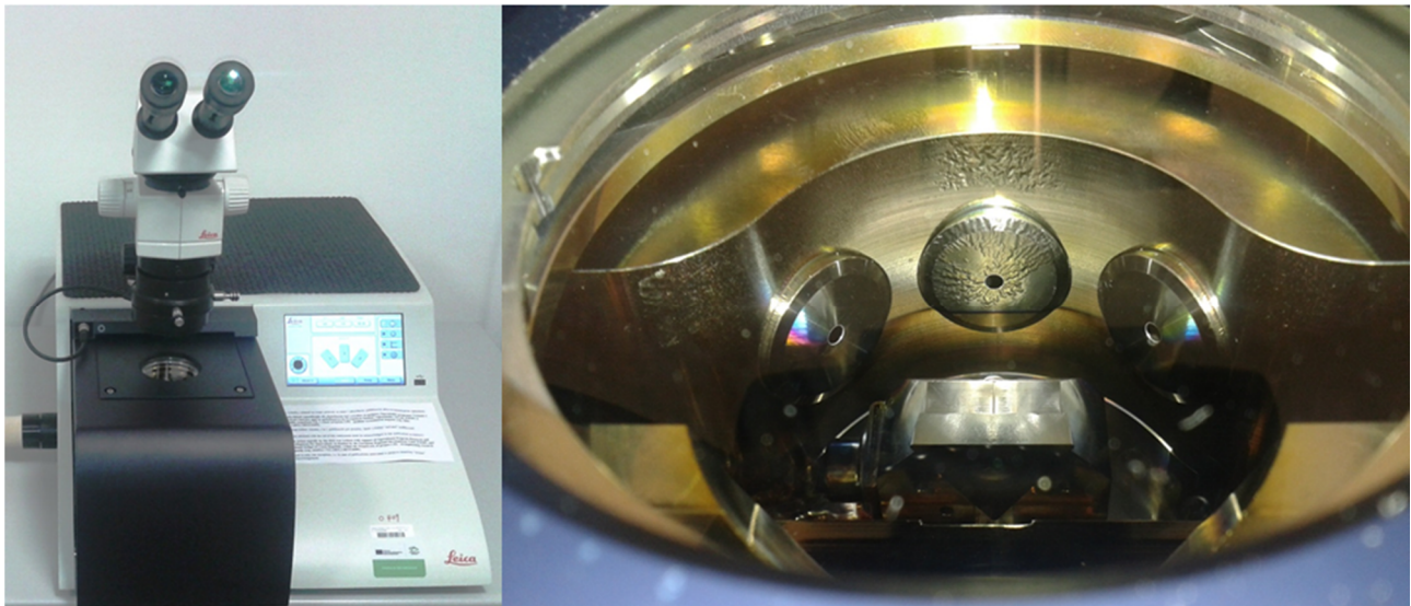
Figure 2 Ion beam milling system Leica EM TIC 3X (right) and the detail of chamber with 3 ion guns (left)
