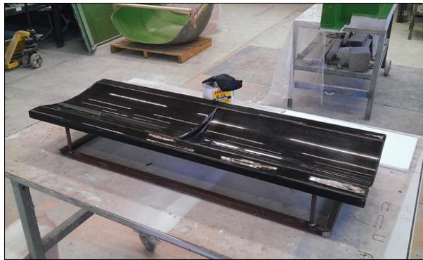
Fig. 2 Prepared manufacturing laminate mold
