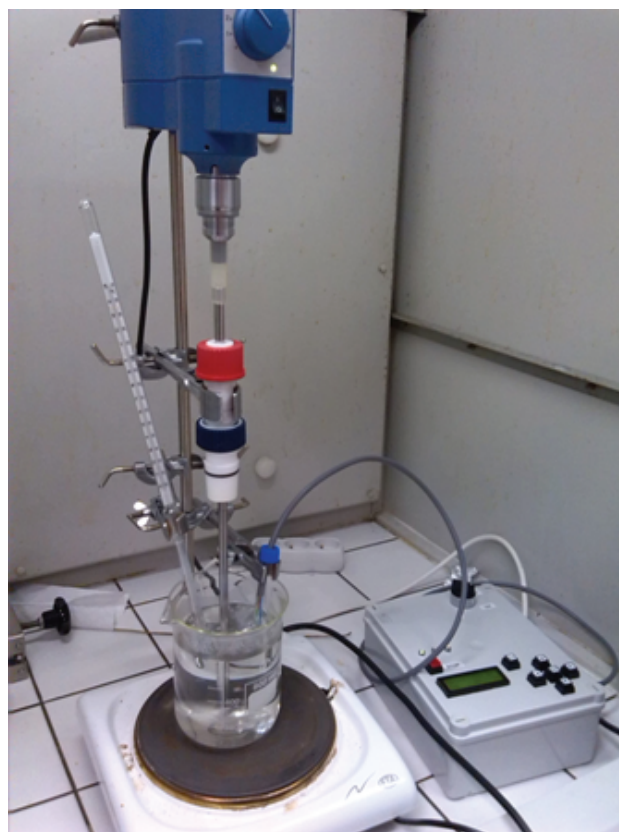
Fig. 9 Setup for measurement of shrinkage of collagen materials
