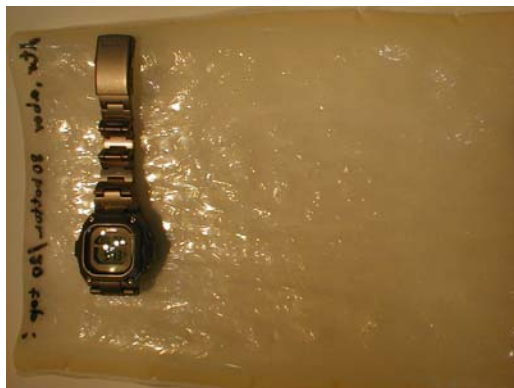
Figure 1 Three layer sheet sample with poor layer distribution and distortion
