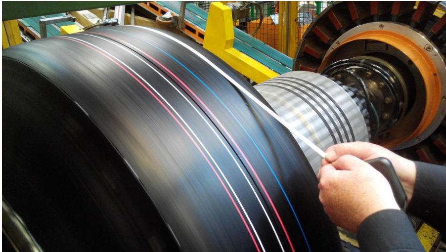
Fig. 1. Current method of circumference measurement of crude tyres.
